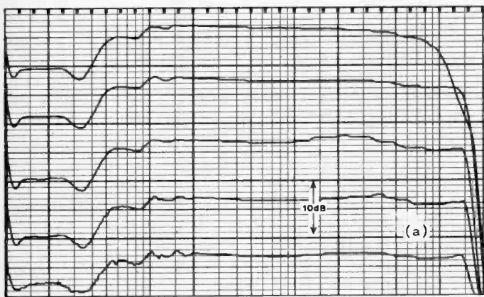
Fig. 8. Tape noise played back via a spectrum analyzer and chart recorder with (a) the Dolby system out, and (b) with it in.
